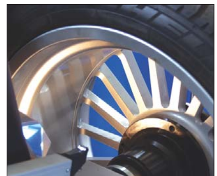
The inner side of the rim is lit up to allow accurate positioning of the adhesive weights.
